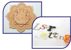
Laser engraving is a procedure that vaporises materials into fumes in order to carve permanent, deep marks. By scraping away layers of the material's surface, the laser beam behaves like a chisel to create marks on the surface. To produce the intense heat necessary for vaporisation, the laser delivers concentrated amounts of energy to specific locations.
